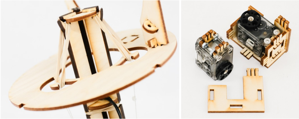
Fig. 7. Detail of the compliant components (elastic bands and strings) used to suspend the head platform (left) and a snap-fit motor mount (right). Snap and press fits are used throughout the structure for ease of assembly and to reduce the amount of required hardware.
